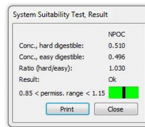
Figure 2. Screenshot of the system suitability test evaluation feature of the vario TOC cube
