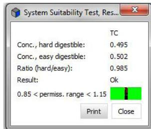
Figure 1. Screenshot of the system suitability test evaluation feature of the **acquray** TOC
