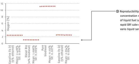
Reproducibility of oxygen concentration measurement of liquid fuel samples using rapid OXY cube equipped with vario liquid sampler (VLS).
